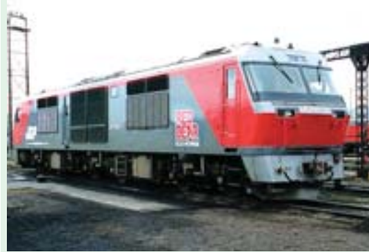
The type DF200 diesel electric locomotive is the first motor-driven train equipped with diesel generators since 1958. It adopted induction motors to realize high acceleration, high speed, and large torque, which resulted in a quick-response generator brake system.
