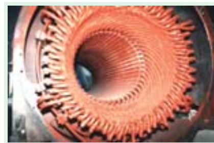
Windings of induction electric motor
