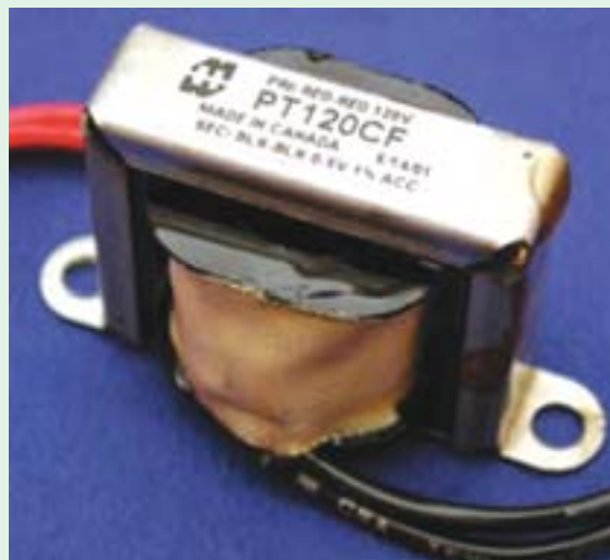
Small Potential transformer
